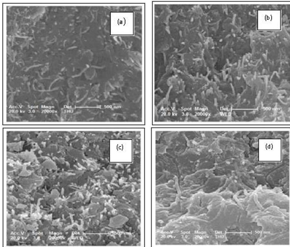
**Figure 4: Scanning Electron Microscopy (SEM) of Fracture Region for Different of Fracture Region for Different SWCNTs Volume Fractions in PFR Matrix at Mag. 20000X: (a) 0.2 Vol.%, (b) 0.4 Vol.%, (c) 0.6 Vol.%, and (d) 0.8 Vol.%**
