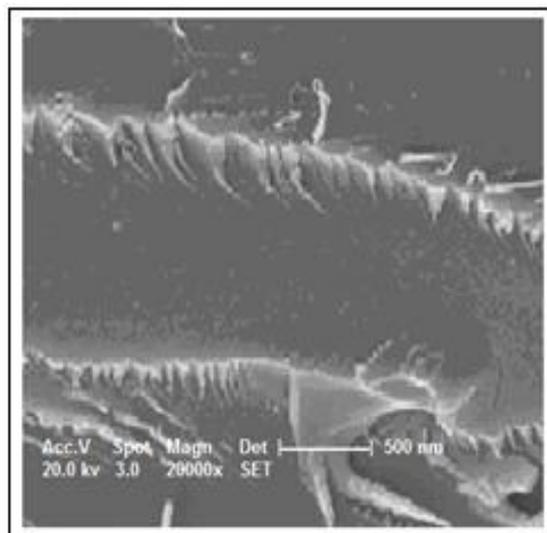
Figure 3: Fracture Surface of Pure Resole Resin Matrix without Reinforcements
