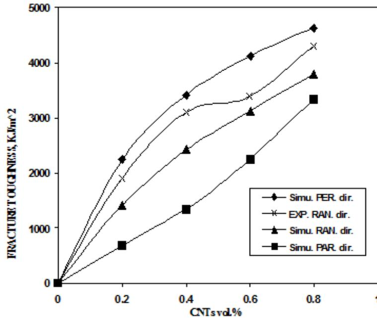
Figure 1: Influence of SWCNTs Vol % and Direction on the Fracture Toughness of Resole of Simulation Results and its Comparison Experimental Random Direction Results
