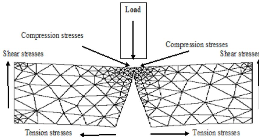
Figure 2: Simulation Load (n) Distribution in SWCNTs Resole Nanocomposite Specimen before Fractured
